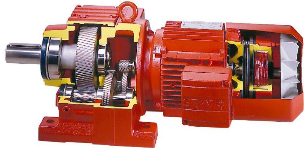
Helical and conic gears have an efficiency of 98-98.5% per stage (1.5-2% loss per stage)
