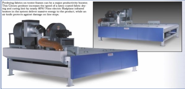
Infrared pre-dryers for textile drying application - Energy reduction – 15% to 20%
