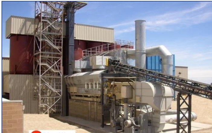
Pre-drying of aggregate using heat from exhaust gases – mixed with outside air to reduce air humidity
