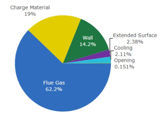
MEASUR or other methods can be used to develop a heat balance for the heating equipment
