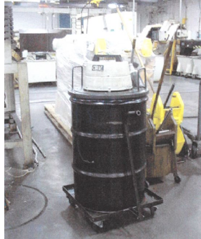
Electric motor-driven vacuum system for cutting fluids. Off, not running $878 year
