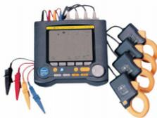
This device helps you directly measure energy consumption, which can be converted into costs. It also logs data to provide electric consumption trends.
