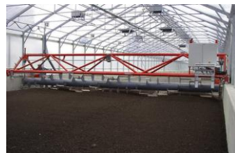
Degremont Heliantis solar drier
