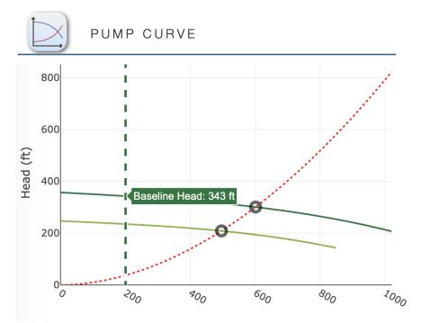
Use pump curve calculator to develop a pump curve and explore the effects of changes in head, flow, pump speed and impeller diameter.
