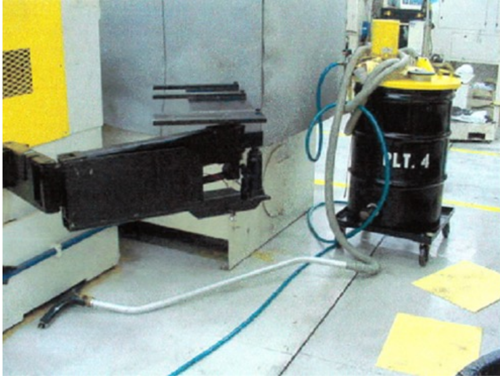
Air-driven vacuum system for cutting fluids, running continuously with machine off – 24/7 operation $6,000 year
