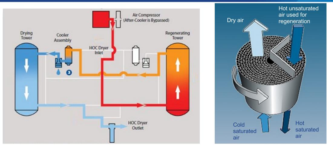
The power requirement, including the effect of pressure drop through the dryer, is approximately 0.80 kW/100 cfm.
