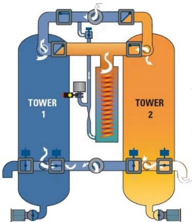
4 hours is a standard cycle: 3 hours drying, 1 hour of regeneration @ 350-400°F
