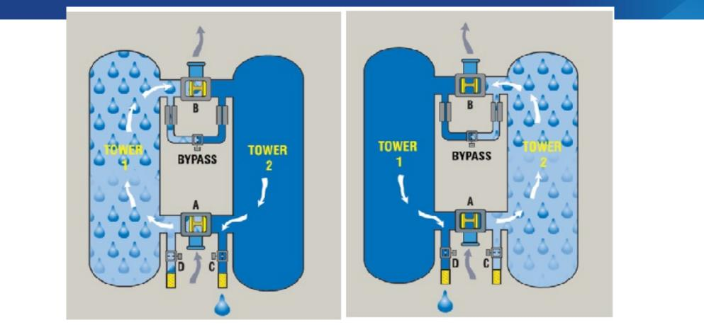
The power requirement, including the effect of pressure drop through the dryer is 2.0-3.0 kW/100cfm.
