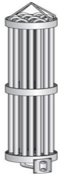
Flue Gas Heat Recovery Tube Bundle
