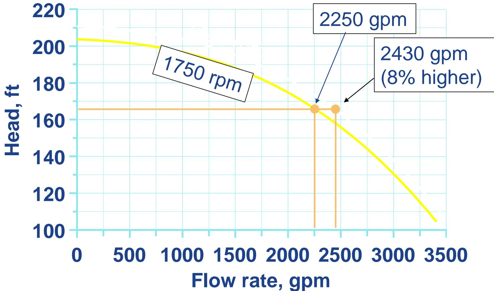
Measured speed is 1780 rpm. The difference is 8% in this case
