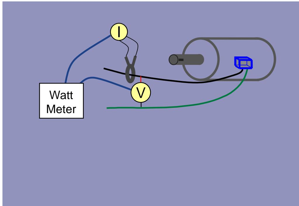
note: the  $V_{\text{rms}}$  above is line to neutral voltage
