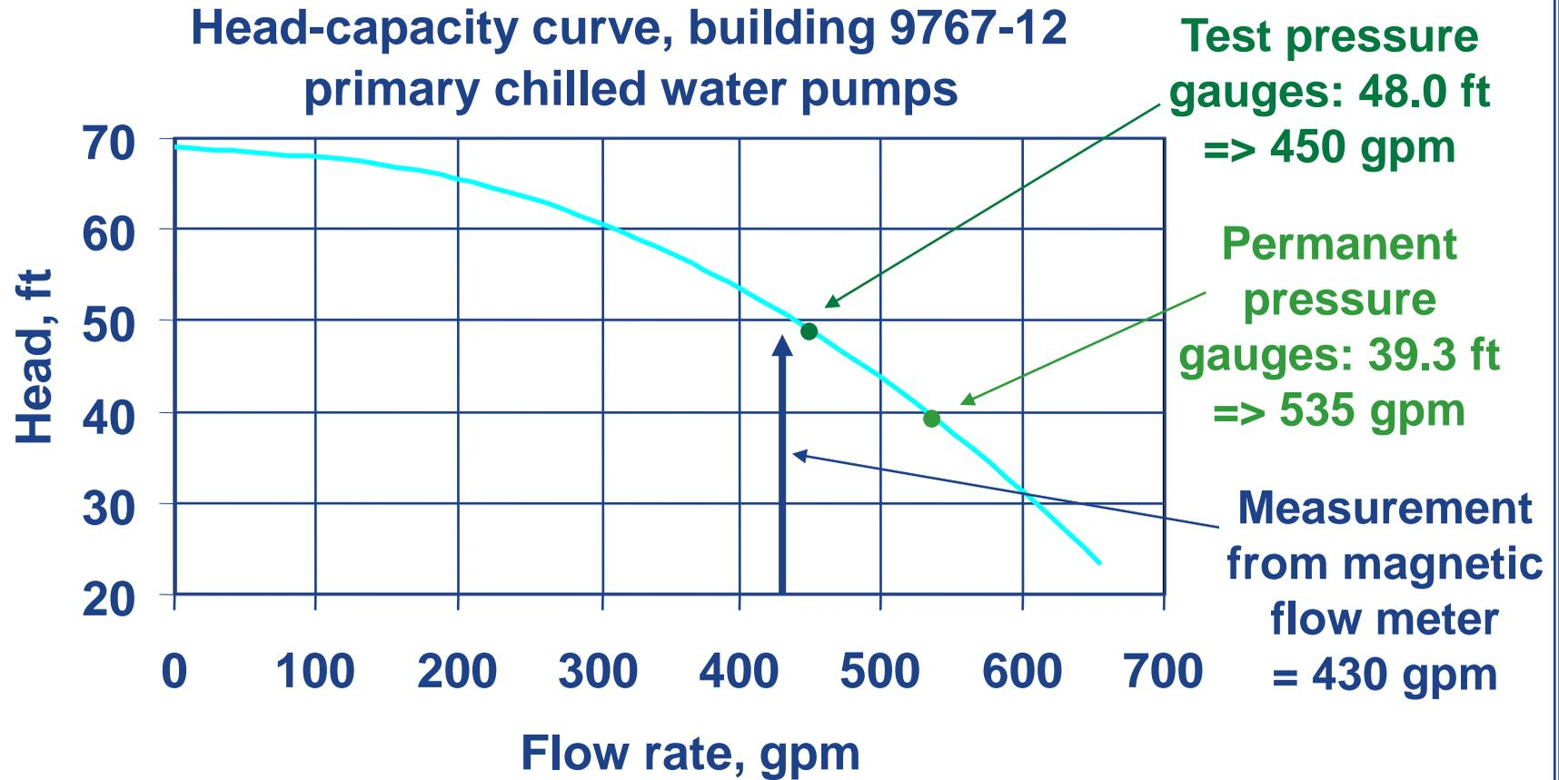
Estimating errors: Permanent gauges + 24%
