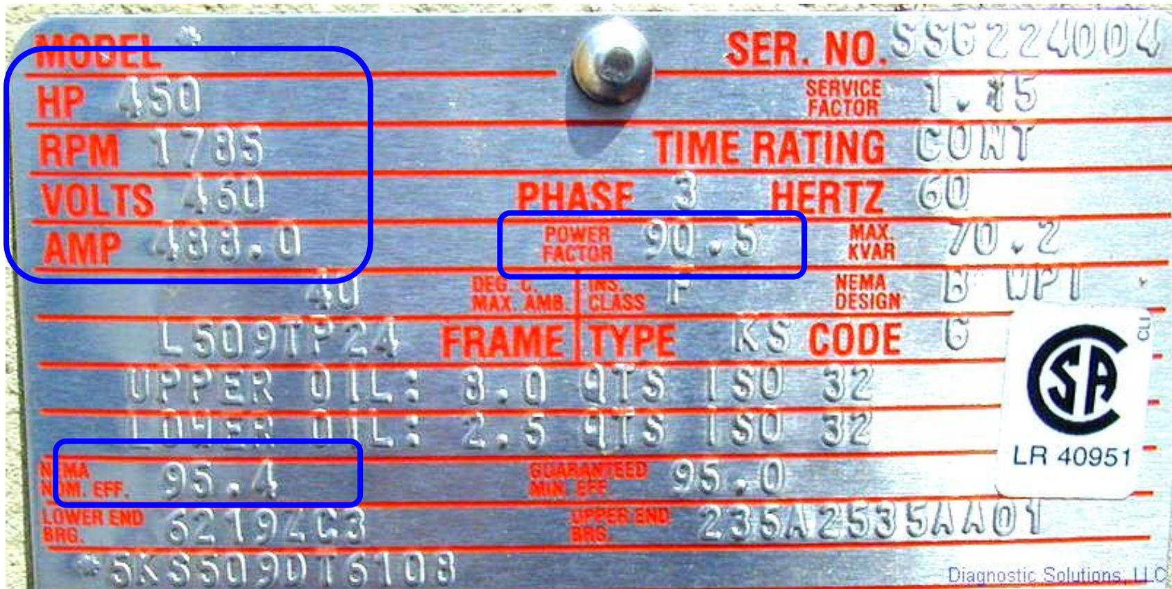
$$\frac{488 \text{ amps} \times 460 \text{ volts} \times \sqrt{3} \times 0.905 \times 0.954}{746 \text{ watts/hp}} = 450 \text{ hp}$$
