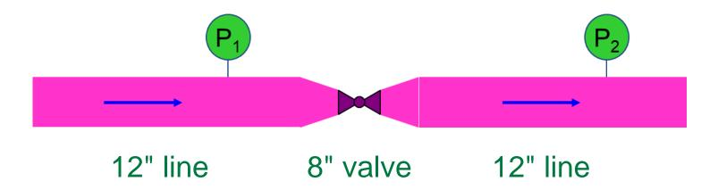
Measured flow rate = 2700 gpm
