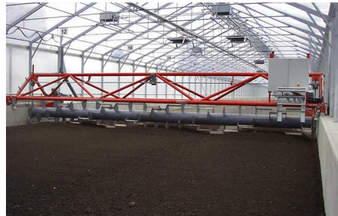
Degremont Heliantis solar drier
