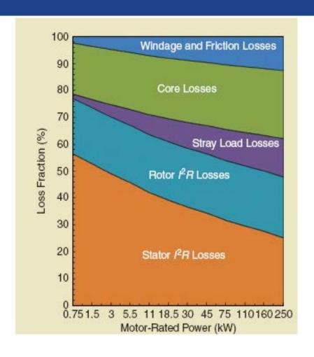
Typical fraction of losses in 50-Hz, four-pole IMs
