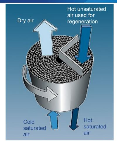
■ The power requirement, including the effect of pressure drop through the dryer, is approximately **0.80 kW/100 cfm**.
