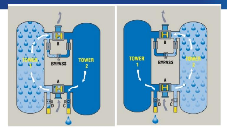
The power requirement, including the effect of pressure drop through the dryer is 2.0-3.0 kW/100cfm.
