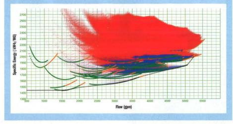
operating limits, represented in Figure 2 by the sand-colored region called the *sandbox*. The lowest point in the sandbox now represents the optimal operating regime for the pump station and is the proverbial needle in the haystack.
