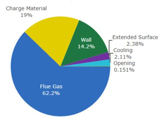
MEASUR or other methods can be used to develop a heat balance for the heating equipment
